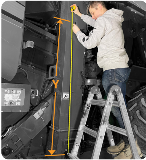
Height (Y) from the center of the bearing to the center of the drill hole
