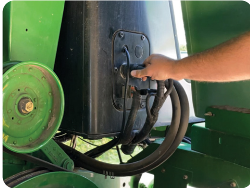
In this install, the harness is routed outside of the cab via a bulkhead below the operator's chair.
